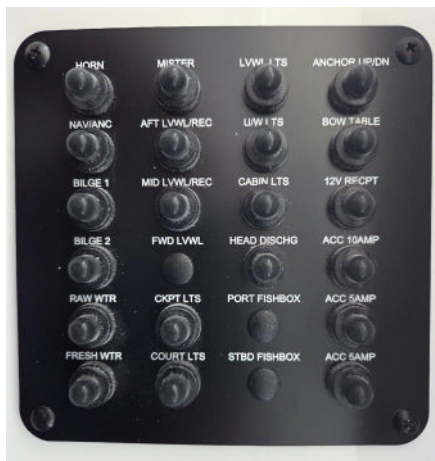
ULTRA 255-305 AND GAMEFISH BATTERY SWITCH AND BREAKER PANELS
