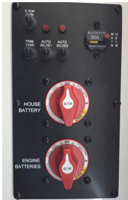
ULTRA 255-305 AND GAMEFISH BATTERY SWITCH AND BREAKER PANELS
